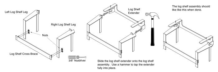
2 Remove the firepot from the pellet stove. Center the log shelf assembly (with extender attached) over the burnpot holder. Replace the burnpot. Place the log on the log shelf extender. When in place the log should appear as shown in the picture below.
